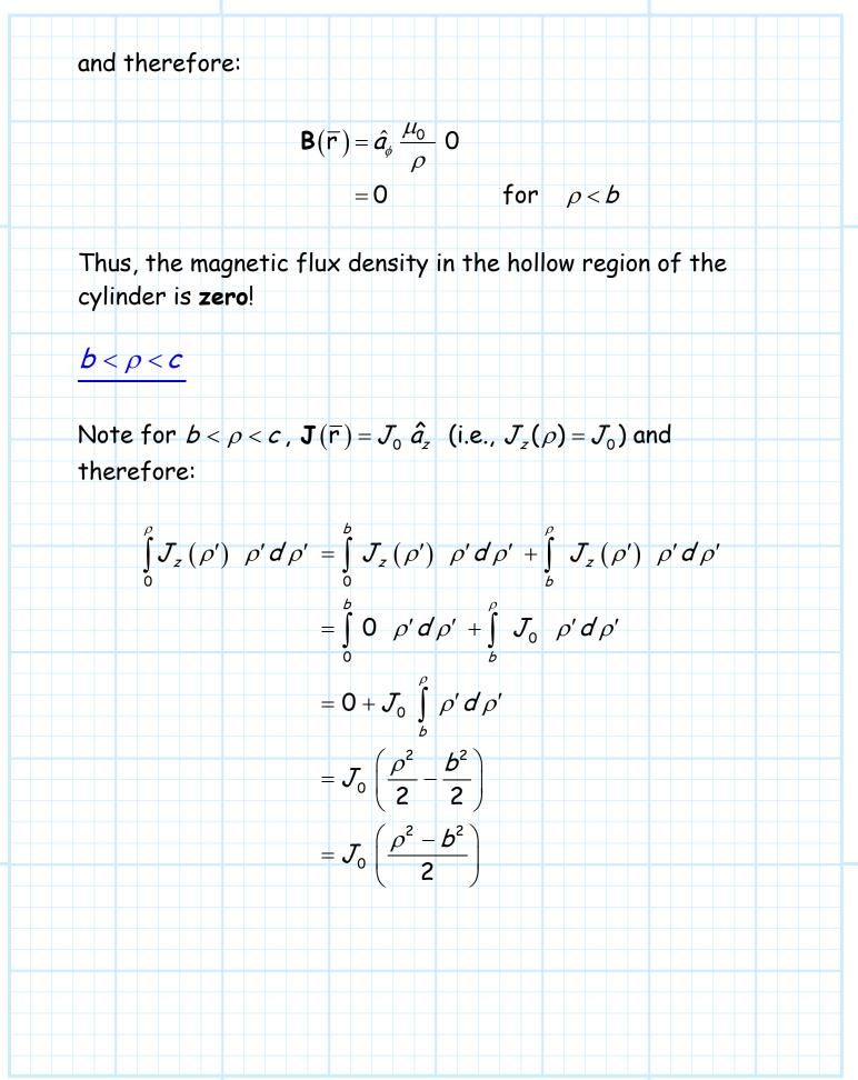
and therefore the magnetic flux density in the non-hollow portion of the cylinder is:
